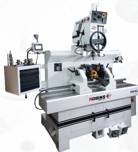
Small Motor Bike Cylinder head in roll fixture on SG8XL
